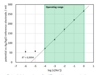
Example output readings for different NaCl solutions
